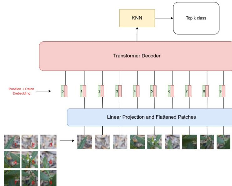
Figure 4: PlantKViT model architecture
