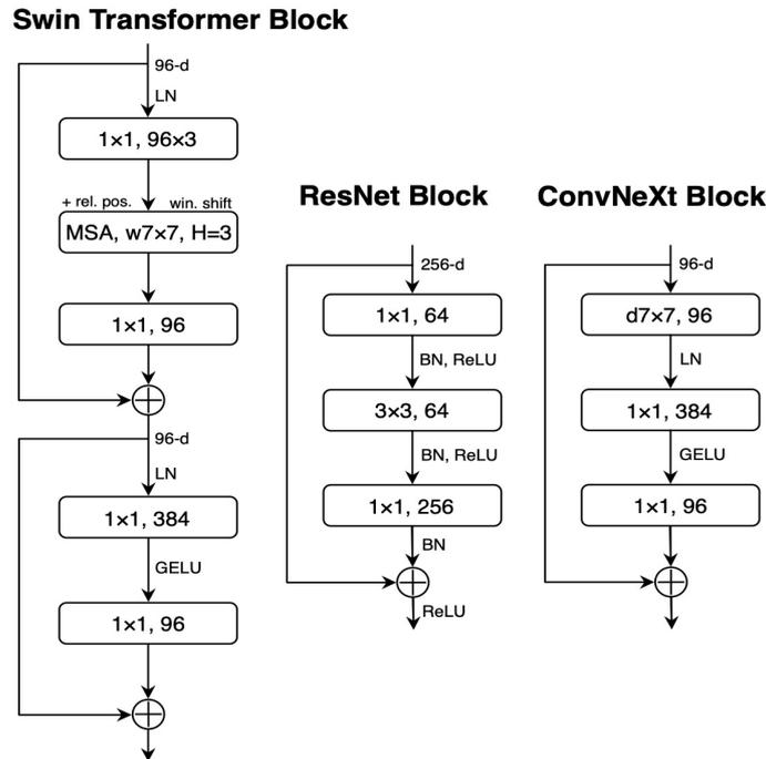
Figure 2: Block architecture of ResNet, Swin Transformer, and ConvNeXt [Liu et al., 2022]
