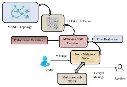
Figure 3: Block diagram for proposed secure data transmission in MANET
