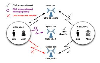
Figure 1: Access control strategy for subscribers based on CSG identity.
