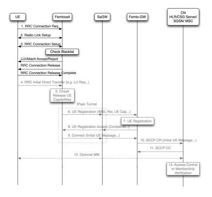
Figure 4: The benefit of auto-reject mechanism. Gray text signifies omitted steps.
