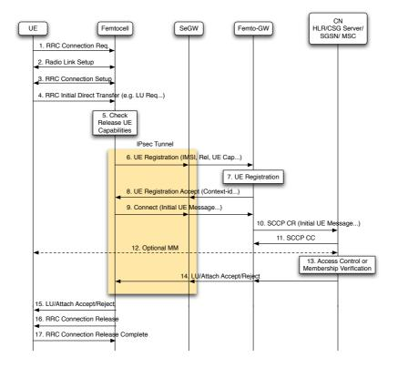
Figure 2: Procedure of UE registration
