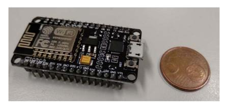
Figure 2: A second generation ESP8266 ESP-12E NodeMCU Amica board.
