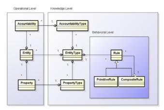
Figure 4: AOM Core Design (adapted from [Yoder et al., 2001]).
