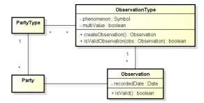
Figure 5: AOM Core Design (adapted from [Yoder et al., 2001]).
