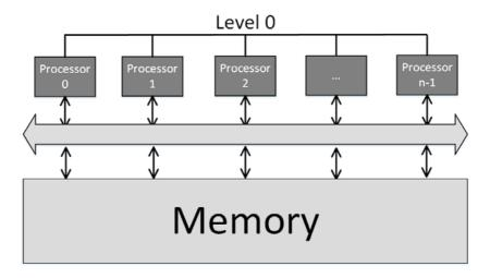
Figure 1: A sample schema of the Parallel Random Access Machine
