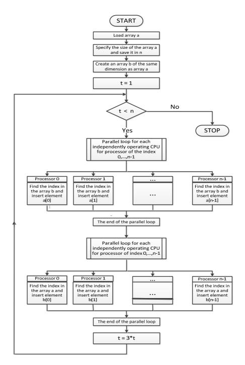
Figure 9: The block diagram of the proposed Parallel Fast Sort Algorithm
