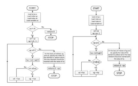
Figure 10: The block diagrams of two functions used in PFSA code implementation to calculate exact position of the insertion, from the left side and from the right side
