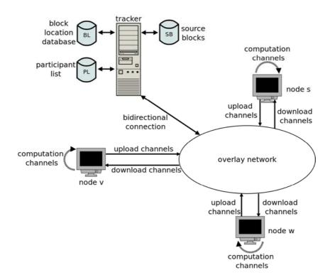
Figure 1: P2P computing system architecture
