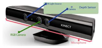
Figure 1: Hardware components of Kinect
