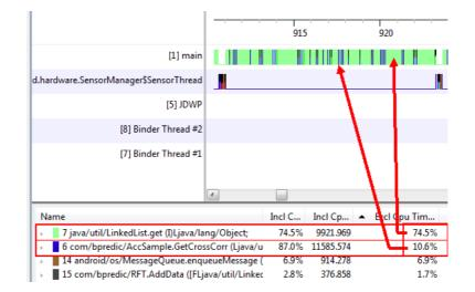
Figure 14: Mobile application profiling results showing functions which are main contributors to CPU load
