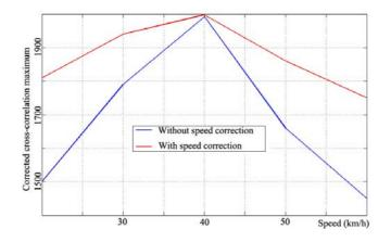
Figure 11: Maximum cross correlation values with (red) and without (blue) speed correction
