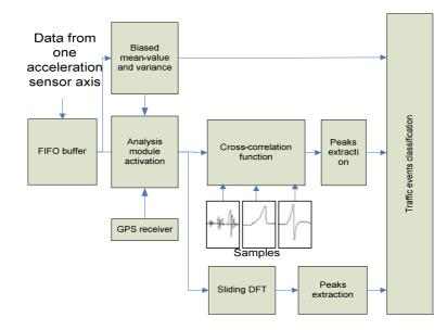
Figure 6: Accelerometer data flow during analysis
