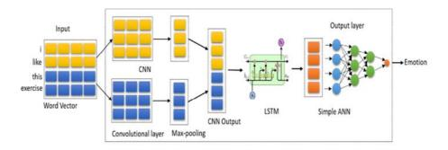
Figure 2: Model 6: DL with CNN and LSTM.
