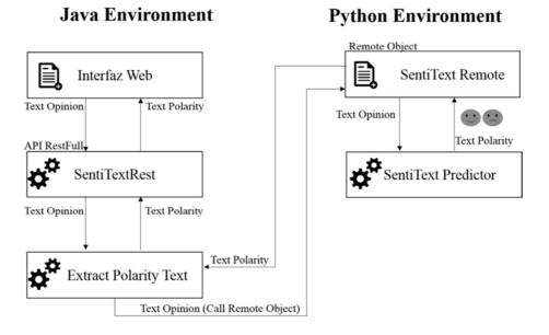
Figure 5: Integration of the DL module into Java Sensei.
