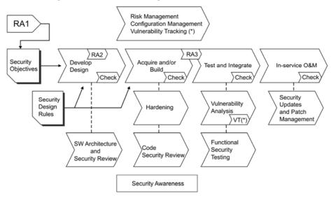
Figure 5: Illustration of Ericsson's RA process in Waterfall SW development.
