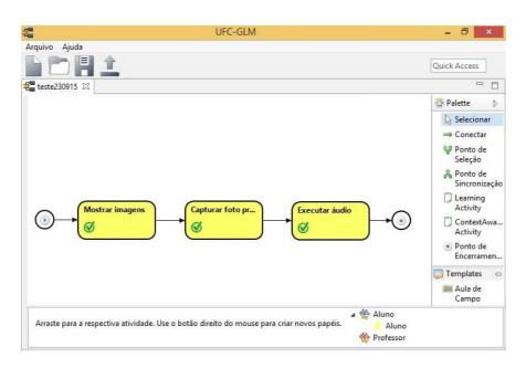
Figure 4: The main screen of the UFC-GLM module. It shows a model with three actions: show images, capture a photo, and play audio
