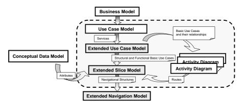
Figure 3: Model-driven process
