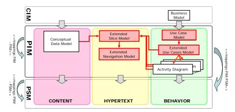
Figure 1: Model-driven framework for WIS development
