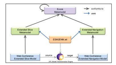
Figure 4: ATL Model Transformation: Extended Slice model to Extended Navigation model
