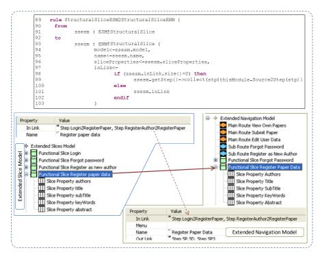
Figure 5: ATL code excerpt and partial views of involved models: mapping Slice objects
