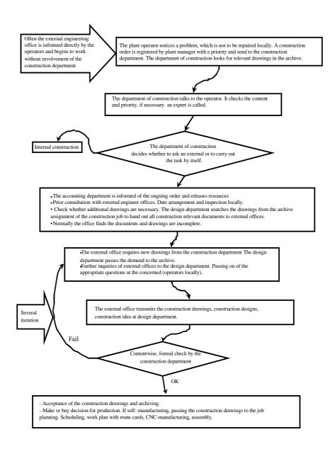
Figure 2: Typical process when constructing
