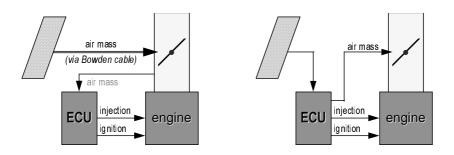
Fig. 1: Traditional Bowden cable solution versus Electronic Throttle Control
