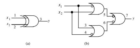
Figure 3. (a) EX-OR gate (b) Its augmented-OR form
