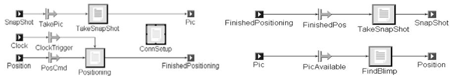
Figure 6: Component models of the camera positioning system
