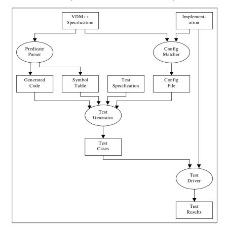
Figure 1: Architecture of the TESTAF
