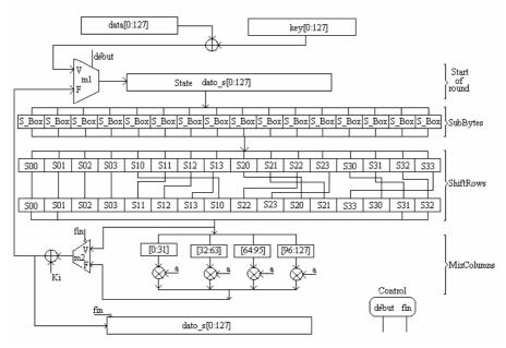
Figure 4: Diagram for the Cipher module
