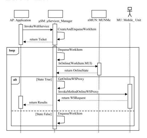
Figure 7: Sequence diagram of a process to create, store and dispatch work items
