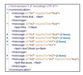
Figure 5: Excerpt of XML specification that defines a set of conversational acts.
