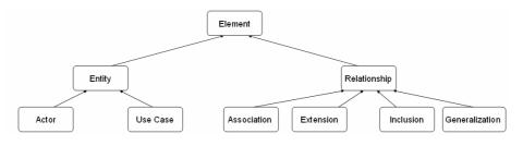
Figure 1: Meta-model of the use case diagrams domain.
