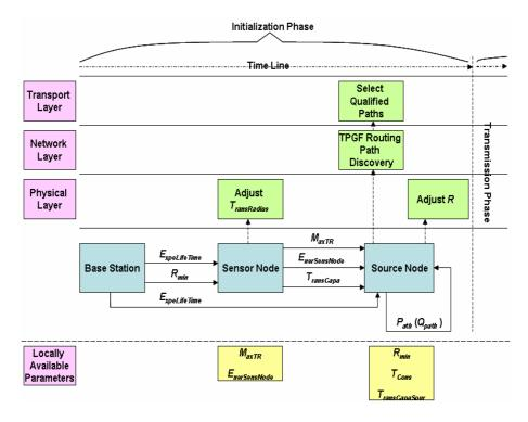
Figure 1: The cross layer framework of RRA scheme
