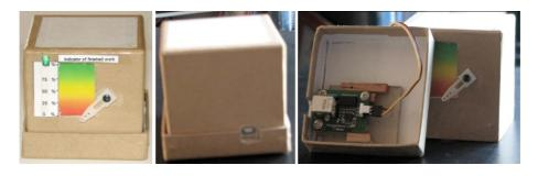
Figure 3: Prototype of the Augmented Object, which use an USB port
