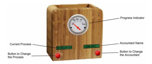
Figure 4: Augmented pencil holder designed for the client
