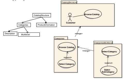
Figure 4: Example of the package merge mechanism applied to use case packages
