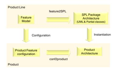
Figure 1: A global vision of the proposed integration of UML with feature models and transformation techniques to manage SPL variability
