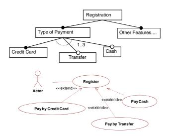
Figure 2: A fragment of a typical SPL feature model (hollow circles represent optional features while filled circles represent mandatory ones), and a use case diagram that applies the extend use case mechanism to represent SPL variability
