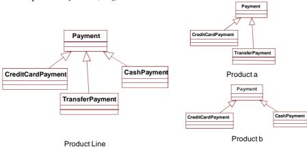
Figure 3: A fragment of an SPL class diagram and two possible derived products
