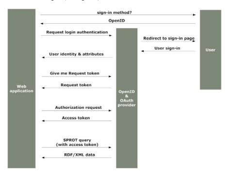
Figure 4: Single sign-on data flow
