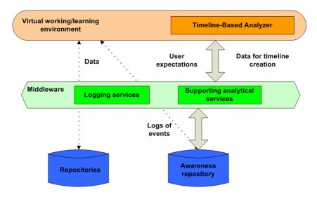
Figure 1: Architecture of TLBA integration with related supporting services.
