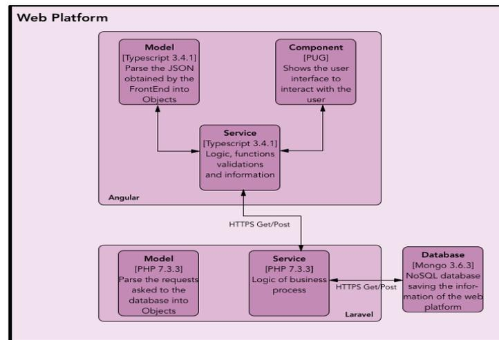
Figure 3: C4 components view of Web Platform
