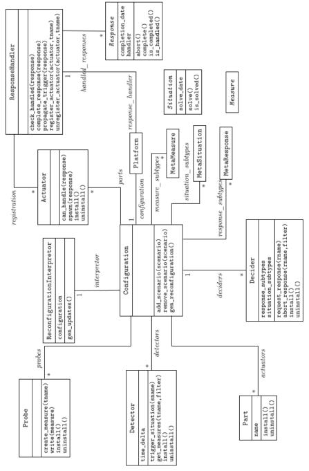
Figure 9: SoREn simplified class diagram
