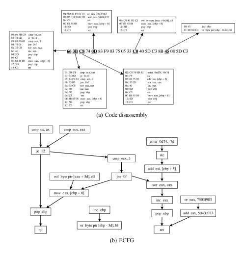
Figure 1: Example of building an ECFG
