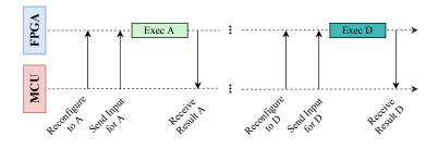
Figure 3: Execution of a Temporal Accelerator on the Elastic Node
