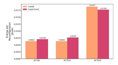
Figure 4: Model prediction vs. preliminary hardware experiment results
