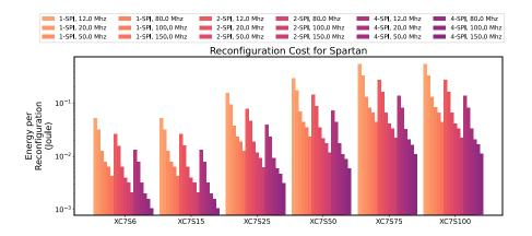
Figure 5: Cost per reconfiguration for chips of the Xilinx Series 7 Spartan family
